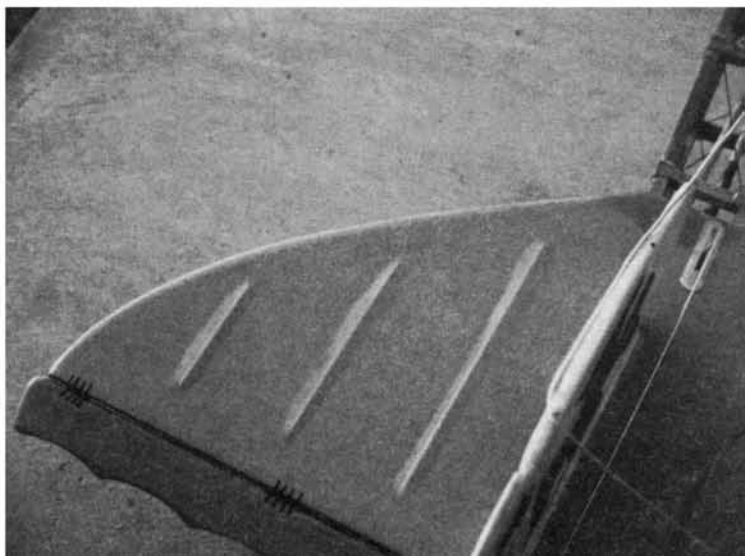
Simulated ribs on stab made from \frac{1}{32} " sq. spruce and covered with tissue.
