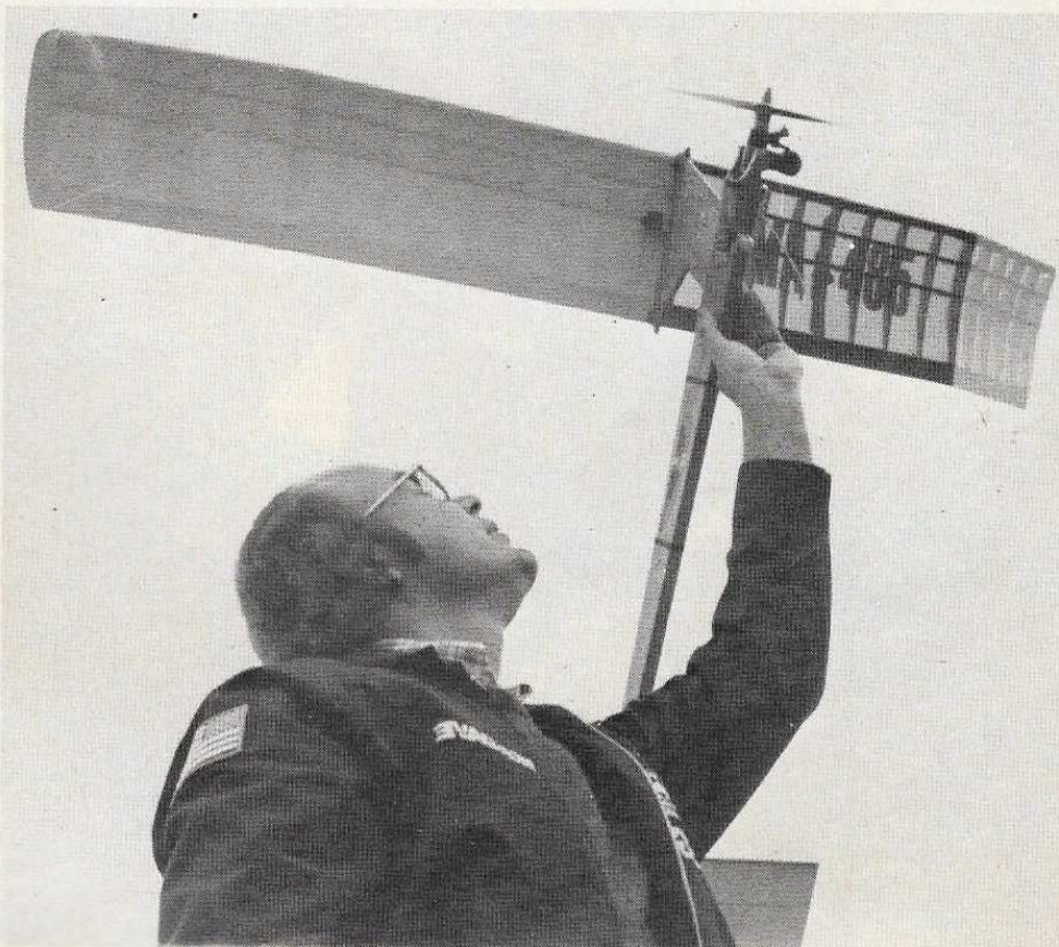
Nose end starts with a plastic Cox 8/4, Cox .15 (old style, not Conquest .15), Tatone Tick-Off, pacifier fuel tank, a 3/32" wire skid. Below: Launch it vertically for an entry into typical pylon spiral climb.
