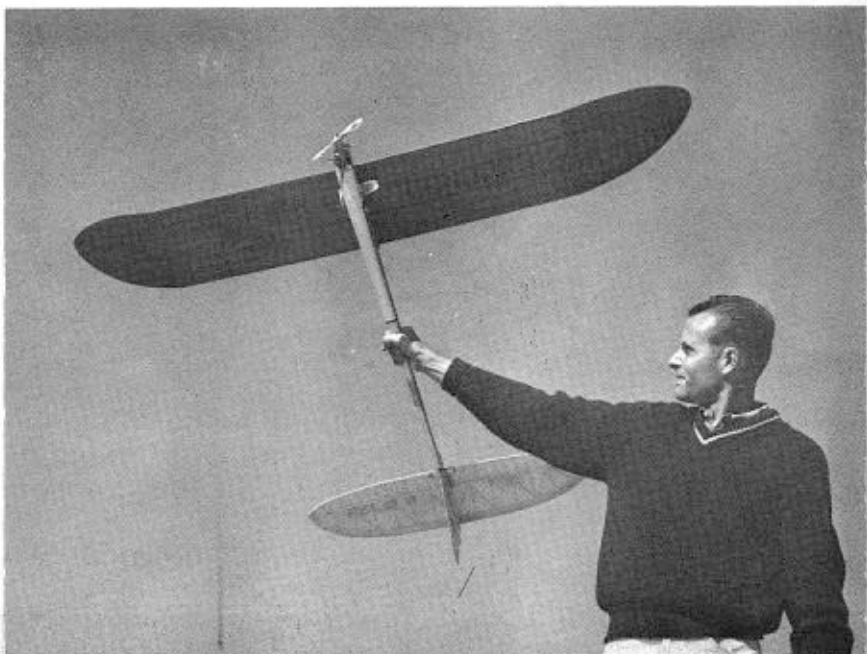
Elliptical tips, undercambered soaring section.
