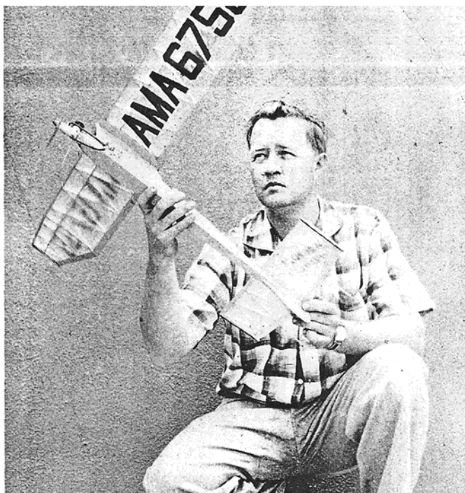
"Lucky" Moody with his original ship. Californian modellers use plenty of dope on their ships. It preserves the models, adding very little weight.
