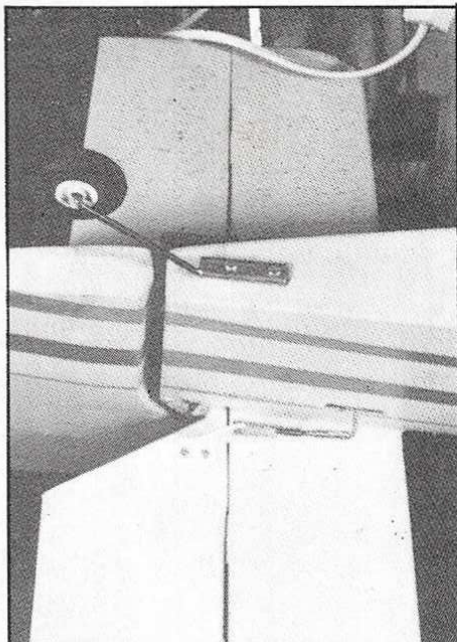
The base of the rudder is thick, hinges must be very strong. Note simple tailwheel bracket which allows quick replacement and could be made steerable.
