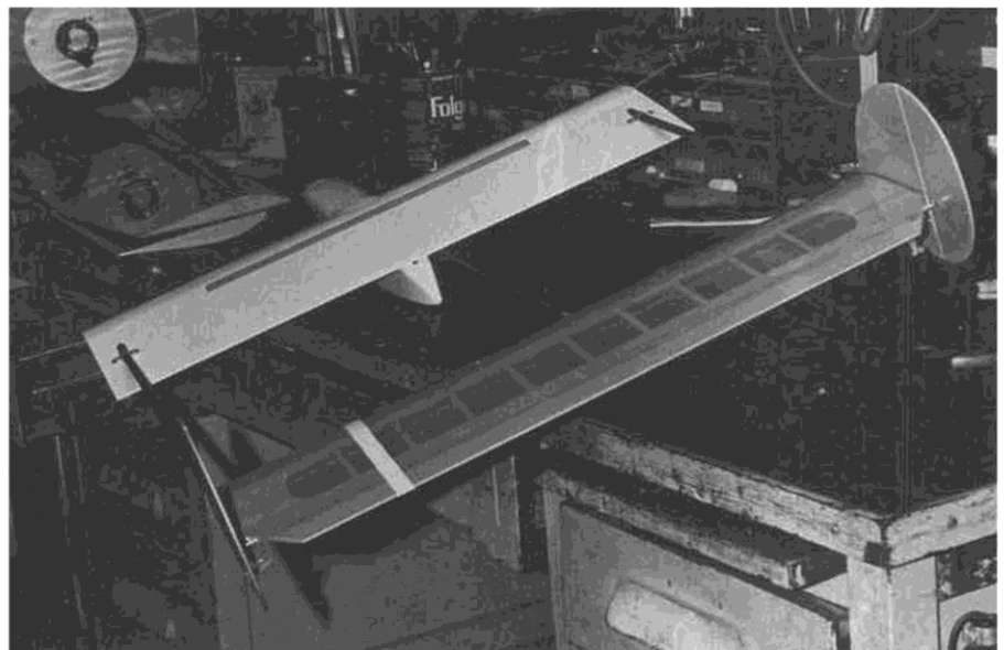
Rear view of Bert's BOOMER. Rudder pushrod comes out left boom, to horn. Tie-rod connects to right rudder. Bert calls attention to his neat, practically NEW work table!
