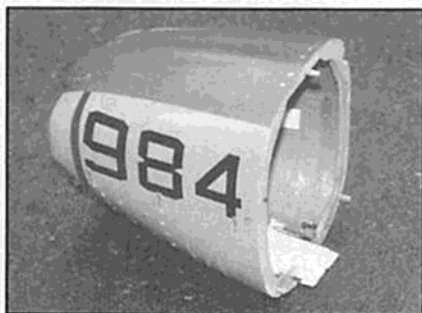
Cowl showing C1, the cowl attachment ring.
