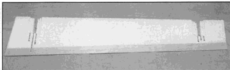
The lower surface of the flap prepared for the flap track and the 1/8" plywood mount.
