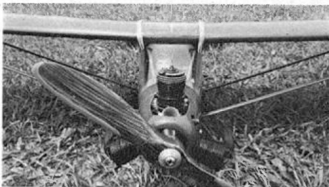
The top view shows the radio installation through the wing bay (above). Two dummy cylinders and a detailed prop add to the scale look (below).
