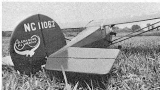
Details of the removeable gear and the control linkages (above). Plenty of rudder and elevator area is apparent here (below).
