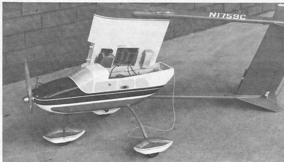
Wing is built in three sections, 2 outer panels and a center panel that support booms.
